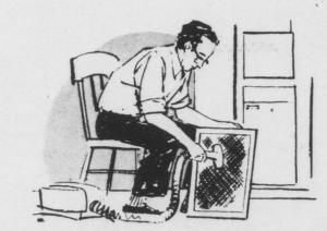
Clean registers, baseboard units or radiators. A thin layer of dust can impair heat radiating ability . . . vacuum cleaning can eliminate the problem.
