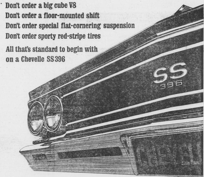
The standard engine in both the Chevelle SS convertible and hardtop is a 396-cubic-inch Turbo-Jet V8 with 325 hp. The standard transmission is a fully synchronized 3-speed with floor-mounted stick shift. (Yes, you can order a 4-speed or Powerglide. Strato-bucket front seats and console, too.) And the SS 396 chassis comes complete with
