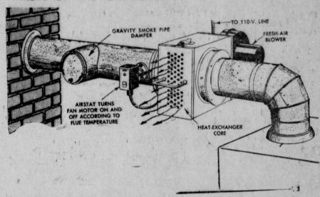
The Hoskinson Free Heater is able to er to heating problem rooms. Gives you extra heat for your playroom, attic, workshop, gaage, or any extra room, yet it doesn't cost a penny more for fuel. In fact you'll save on fuel by keeping cold rooms properly heated. Phone or Write For A Heating Engineer. He will be Happy To Explain The FREE HEATER At No Oblibation To You.
