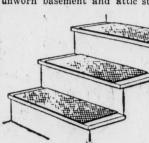
cover the slippery surface with some Masonite Tempered Presdwood one-quarter inch thick. Nail it down with the rough, screen side up, thus successfully skid-proofing the stairs.
