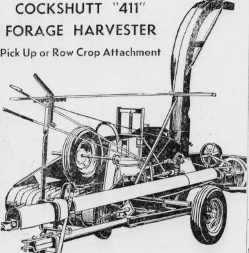
Row crop model has plenty capacity for all heavy yielding corn and row crop silages. Wide throat and three gathering chains make it possible to harvest storm tangled crops. Cutting height is quickly adjustable. nake it possible do like the second s
