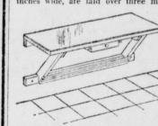
base for the top. For a tough working surface, nail over the planks a piece of Masonite quarter-inch tempered hardboard, the material widely used for bench tops in factories because it "has what it takes"
