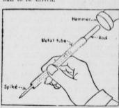
Now take an iron rod which fits loose ly in the tube. This rod should be square at both ends.
