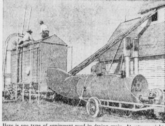
Here is one type of equipment used in drying grain. At extreme right is inclined plane elevator to transport dry grain from drying bin to storage loft.
