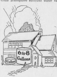
The Water Pan in Old Style Heating Plants Holds a Gallon of Water, More or Less, and Usually Is Dry. Six to Eight Gallons of Water Average Size Home During the Win-
