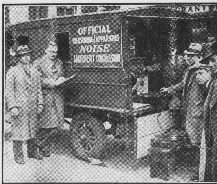
Technicians from the Bell Telephone Laboratories are shown measuring the deafening effects of noise in New York, in connection with studies being made by the Noise Abatement Commission. A microphone records the city's harsh cacophony is suspended around the neck of the man to the left. The telephone engineer at the rear of the truck, holding a receiver to his ear, is measuring and charting the intensity of the din.
