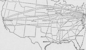
The above map shows the twenty-nine cities which the Radio Corporation of America hopes to include in an inland radio telegraph network soon. Work already is under way to give radio telegraph service to fourteen of the citles, on wave lengths already granted. These stations will be at New Orleans, Kansas City, Detroit, Cleveland, Chicago, Los Angeles, Seattle, Denver, St. Louis, Cincinnati, New York, San Francisco, Boston and Washington.
