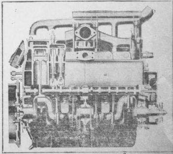
In the new Essex, the development of the power plant into an engine delivering 70 miles an hour maximum and 60 miles an hour all day long has led, among other features, to the adoption of new main and connecting rod bearings on which patent applications are pending.
