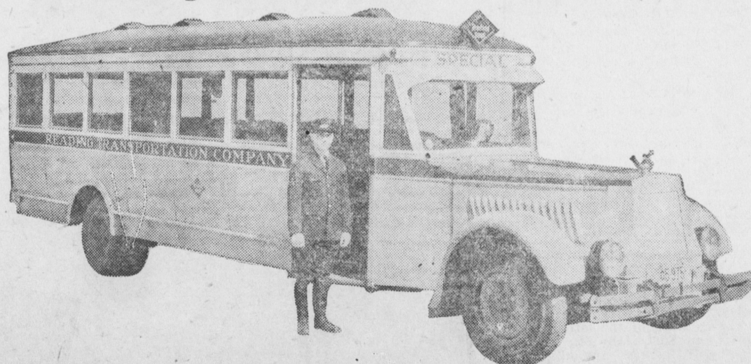
Specially designed motorcoach of the Reading Transportation Company, a subsidiary of the Reading Railroad, which has been adopted for use in the new steam-motorcoach co-ordinated service throughout eastern Pennsylvania. The motorcoach is 30 feet in length and has seating capacity for 29 passengers. Head-rooms of 74 inches. Individual reading lights set in overhead parcel racks are a unique feature. The seats are covered with Spanish leather and the coach affords the comforts of a parlor car.
