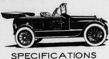
MOTOR—Sis cylinder, cast singly, bore 4 inches; stroke 41 inches; seven bearing crank shaft; en-ed values, easily adjusted and removed engine develops 48 horse power.
