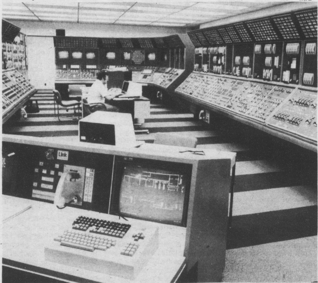
The simulator at the Susquehanna Training Center is a duplicate of that portion of the Susquehanna nuclear power plant's control room which controls Unit 1 and systems common to both of the plant's nuclear reactors.
