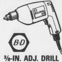
Variable speed—the farther you pull the trigger, the faster the drill's speed. Double-reduction gearing; double-insulated 1/3-hp motor. Drills 3/8" steel, 3/4" hardwood. 45/7180 @
