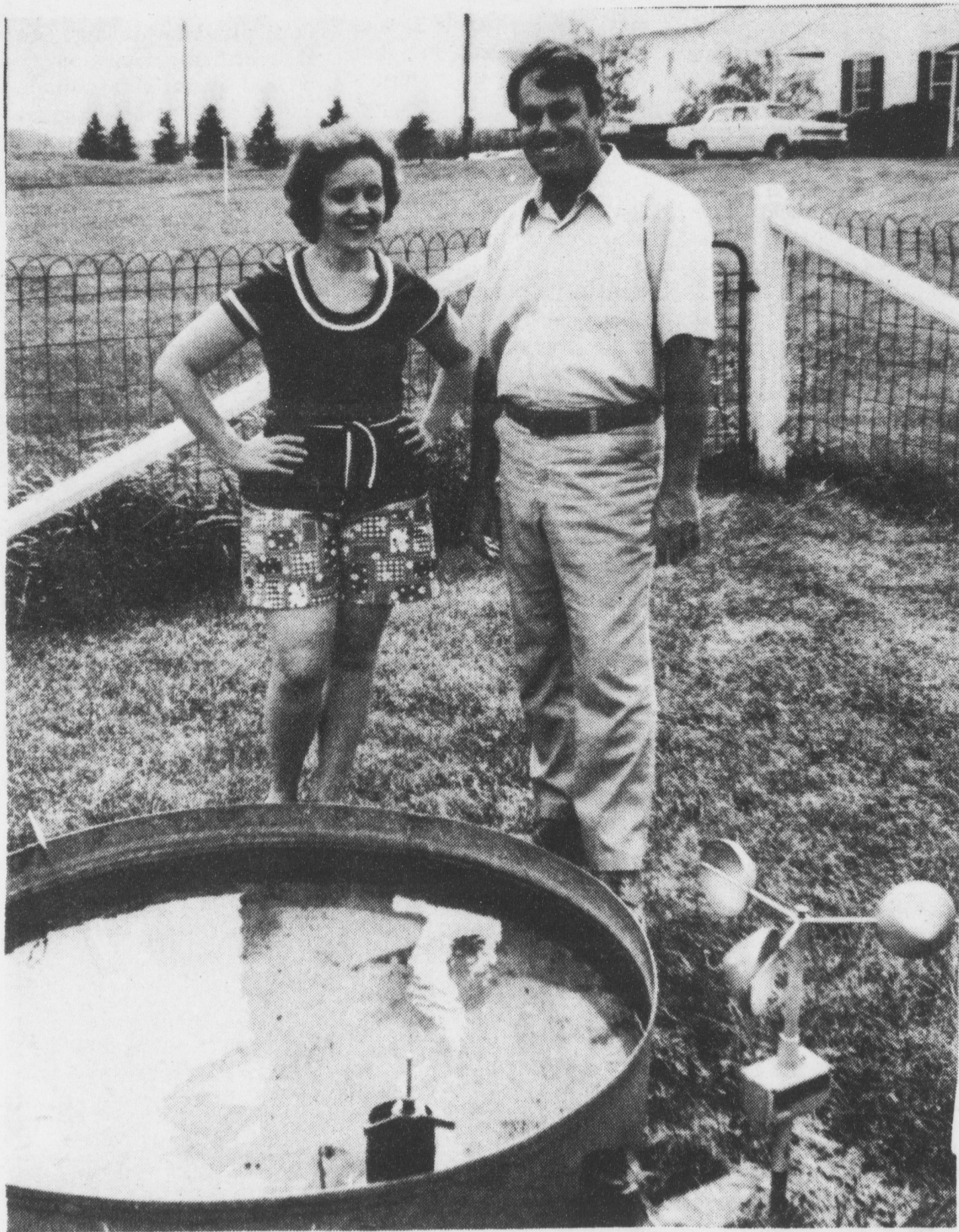
John and Sandra Yocum pose with the evaporation meter in their weather station. The meter simply allows measurement of how far the level has fallen.
