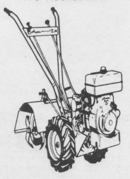
The Ariens 7 H.P. Rocket is a front mounted engine tiller with two speeds forward and two reverse plus swing handlebars, the Ariens Rocket will let you handle all jobs with ease.
