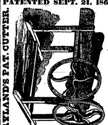
The merits of this Machine consist, in part, in the attachment of curved knives to the arms of the cuting-wheel, the shearing cut across the mouth-piece the great power and directness of the blow, by which treble the volume of material is cut, with less power than is required by any other Macnine; those combined with its durability and simplicity of con-
