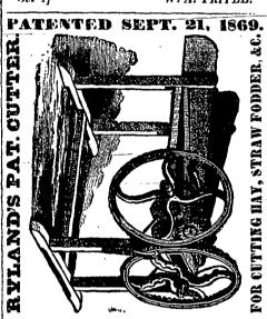
The merits of this Machine consist, in part, in the attachment of curved knives to the arms of the cutting-wheel, the shearing cut across the mouth-piece, the great power and directness of the blow, by which treble the volume of material is cut, with less power than is required by any other Machine; those combined with its durability and simplicity of con-struction, command public attention. Nothing liable to get out of order, but what a boy could remedy
