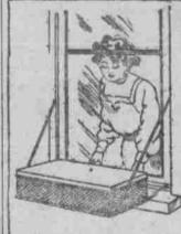
each end and rods running up to the side of the window to further strengthen its position. The box is made of wire gause with a solid lid, thus permitting a free current of air through it, yet protecting the con-
