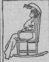
winding shaft and clutch and a ratchet, the last named operated by rock arms pivoted in one of the rock-ers of the chair. As the chair rocks forward the ratchet is moved one way and turns the gearing which in turn operates the driving shaft and makes the fan revolve. When the turned in the opposite direction and the whole movement is reversed. Thus a steady current of air is kept
