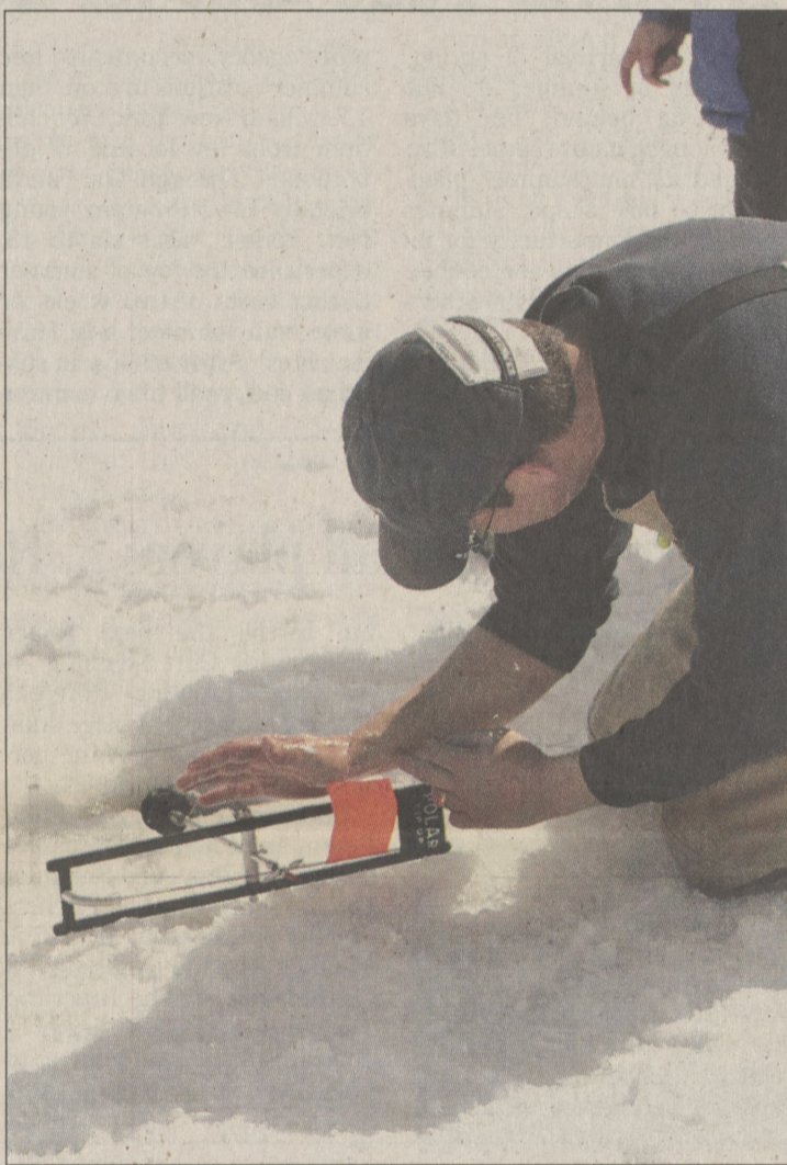
Measuring against an ice popper, Michael Barber estimates the ice thickness at 8-9 inches.
