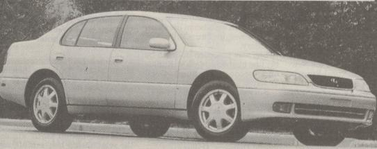
220 HP IN-Line 6 Cylinder 4 Wheel Anti-Lock Brakes
