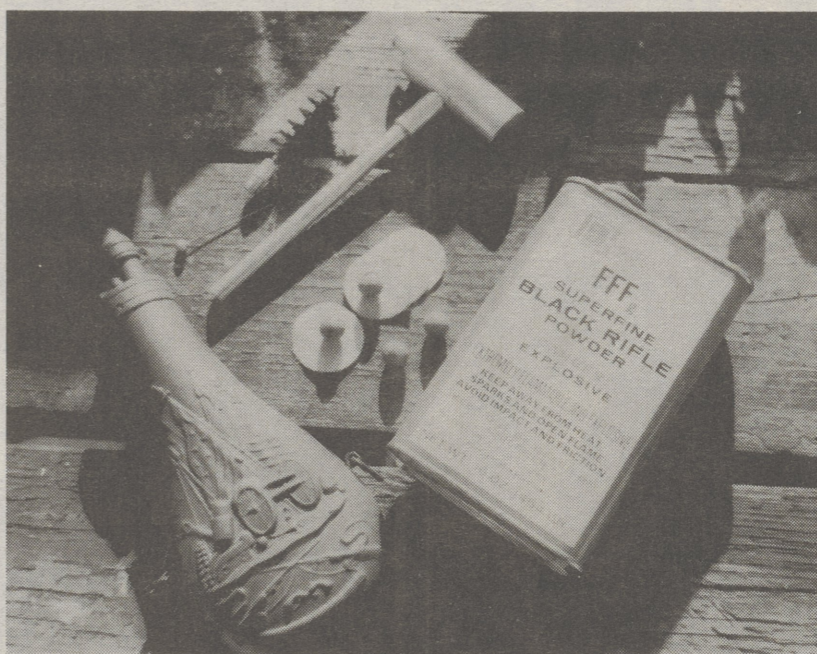
THE RIGHT STUFF —These items should be part of every black powder shooter's basic equipment kit: clockwise from right: black powder, powder flask, a pin to clean the torch hole, cleaning brush for the barrel, ball starter, lubricated patch and round lead shot. (Post photo/Grace R. Dove)
