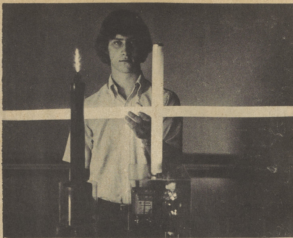
MODERN SCIENTIST—Gordon Davies of Dallas is definitely not your 'modern scientist' but has demonstrated an extraordinary talent in the fields of electronics and engineering. Davies is pictured above with his Tesla Coil, a device which emits 60,000 volts of high frequency current, at a frequency of 500,000 cycles per second. Today, energy transmitting machines are used in the heat treating of metals and in hospital operating rooms as a means of cauterization.
