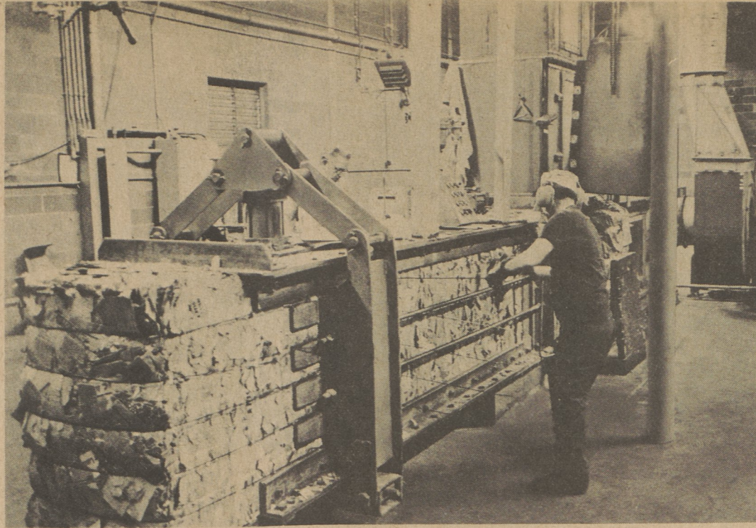
Acme Markets, Inc., which operates over 600 supermarkets in seven eastern states, doesn't burn its waste paper and cardboard, which would contribute to air pollution. Instead, it prepares this material for recycling by paper manufacturers. Above, employees at one of Acme's Philadelphia-area warehouses operate huge shredder and baler which compresses the waste into half-ton bales for shipment to paper makers.
