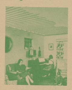
Chromalox Ceiling Thermwire provides a completely hidden heat source. Simply staple to the ceiling lath and cover with plaster. It can be used anywhere, in either dry wall or plastered ceilings. Automatic control is supplied by line or low voltage room thermostats. room thermostats.
