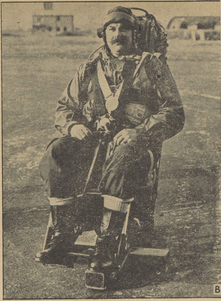
IN THE EJECTION SEAT he was testing when he was shot from a Meteor jet aircraft at 29,000 ft. (about 5 1/2 miles) up over Oxfordshire, England, is Parachutist Bernard Lynch. The new seat of the British Martin-Baker Aircraft Co. automatically allows the pilot to escape from high-speed aircraft at high or very low altitudes. An earlier Martin-Baker seat, standard fitting of Britain's Royal Air Force, has been adopted by the U. S. Government.
