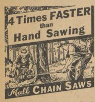
The powerful, lightweight Mall Model 7 Chain Saw is the faster, easier way to cut cordwood, clear land and fell, buck and limb large and small timber. Automatic clutch prevents stalling engine. Engine starts easily in all kinds of weather—uses very little fuel. All controls are located on the handle bars for ease of operation. Chain may be indexed for angle cuts. The Model 7 Chain Saw is a completely self contained unit that may be carried wherever man can walk.
