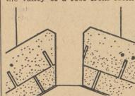
ing the corners of asphalt shin gles and penetrating behind the roofing material, cut off the points as shown in the sketch. This will direct the flowing water into the valley, which will carry it harmlessly into the roof gutter.
