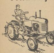
With the Pony you handle your work in just a fraction of the time it takes with horses or hand-operated tools. You're up on a comfortable seat where you can see what you're doing all of the time. The Pony handles easily—turns in an 8-foot radius. Convenience is built into Pony - handy controls and automotive type dash make driving simplicity itself.
