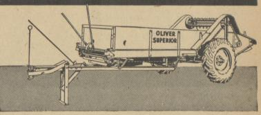
To get the fullest value from manure, it should be spread thin. The Oliver Superior No. 7-AW spreads as little as four loads per acre, and the Hammer Mill Wide Spread cuts and smashes the manure to uniform fineness . . . distributes it evenly over a 7-foot swath.
