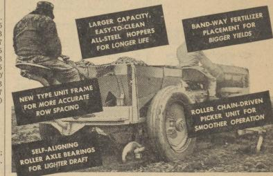
THIS lighter draft Farquhar Iron Age Planter assures you even greater accuracy, flexibility, no matter what your acreage! Has self-aligning roller bearing axles for lighter draft; rigid construction for greater planting accuracy. Easy to clean, reinforced all-steel hoppers plus exclusive Band-Way fertilizer placement that assures greater yields!
