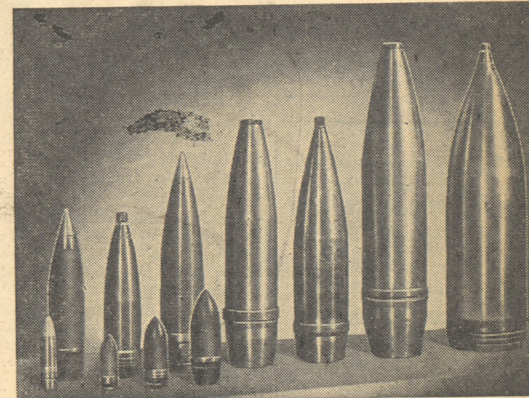
Here are a few of the shells made in Canada: Front row—40 mm ack-ack; 37 mm 6-pounder, and 75 mm anti-tank. Back row—25-pounder; 3.7-inch anti-aircraft; 4.5-inch; 6-inch howitzer; 5.5-inch; 7.2-inch howitzer, and 9.2-inch howitzer.
