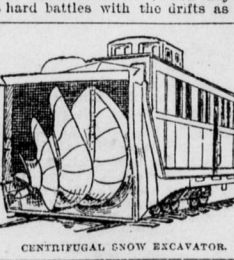
CENTRIFUGAL SNOW EXCAVATOR.
