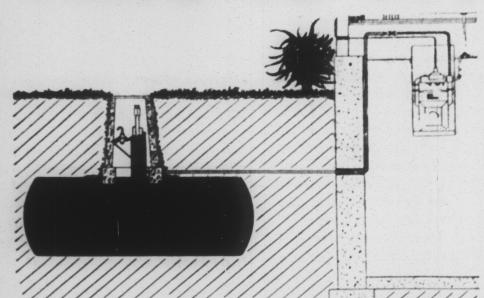
The underground, metered system which supplies GAS SERVICE for cooking, heating water and refrigeration in homes, commercial or industrial establishments beyond the reach of city pipeline
