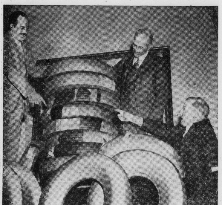
Here are members of the house interstate commerce committee as they inspected 18 retread tires developed under a new process which will provide immediate solution to America's tire problem. The tires, called "Victory Camel-Back," were made under government supervision with five pounds of reclaimed scrap rubber and two ounces of crude rubber.
