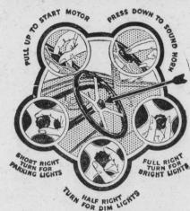
A single button, conveniently located in the center of the steering wheel, controls all functions of starting the motor, operating the lights and sounding the horn. This does away with all troublesome foot fumbling for the starting button. It also avoids changing from the comfortable driving position to reach & light switch on the dash. With the new "Finger-Tip Control," you can at all times keep your hands on the wheel and your eyes on the road—an important aid to safety.
