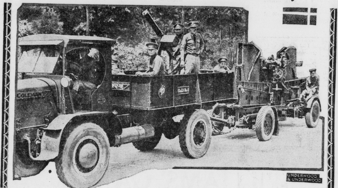
A new type of antiaircraft gun has been developed to protect the army's recently motorized force from aerial attack while on the road. The gun is drawn by a fast four-wheel drive truck and is capable of being fired while in motion.
