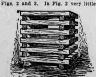
room is taken up, and at the same time individual pieces of timber touch at very few points, thus permitting air circulation on all sides of the wood. When quick drying and seasoning is wanted, Fig. 3 shows a better method and the one commonly employed.
