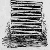
small dimension lumber. Inch strips for edgings are placed near each end, and in the middle of the pile. top course of boards is put on in the form of a roof to shed the water. Very useful methods of piling ties, posts and other timber are shown in
