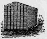
space between the pieces, but in the arid regions it should be piled closer to prevent too quickly drying out and consequent checking of the wood. Fig. 1 shows a very satisfactory method of piling boards, planks and
