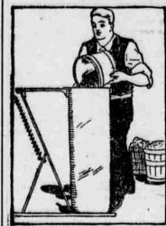
man, and is shown in the accompanying illustration. The sack or bag holder comprises a suitable platform, on which are mounted inclined standards, by which the bag is braced. At the top is a lever which is hinged to one of the uprights. At the end of the lever are two rings, one fitting within the other, the bag being clamped within them. A spring at the rear serves to hold the lever supporting the rings, thus supporting the bag in an upright position.
