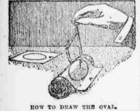
compasses would draw on a flat surface if opened to the same extent. The breadth of the oval will depend on the size of the cylinder used.
