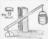
beam. First the weight draws up the edg for scale; the formula for making, and the carenes marred as little as bucket. Water running into the bucket however, must be nicely observed. The fills it, and its weight carries it down, lifting the weighted end. When it full of the mixture, requiring three strikes the ground, the valve is forced up, letting the water out. Relieved of merged as they pass along. A second his weight the bucket rises, only to fill and descend again.
