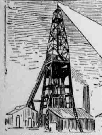
KIMBERLEY SEARCHLIGHT. (A powerful electric light is installed on the shaft head at the De Beers mine. By this light signals were exchanged between Kimberley and the force under Lord Methuen.)
