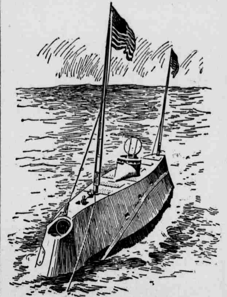
BOW VIEW OF THE "HOLLAND." (The mouth of the aerial torpedo gun, the superstructure deck and conning tower are shown.)
