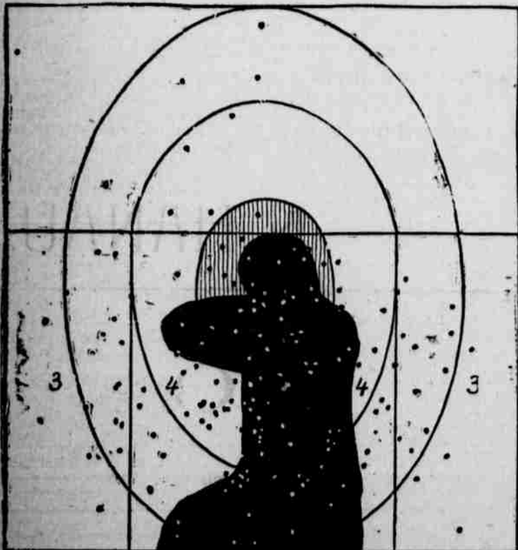
500 AND 600 YARDS TARGET, SHOWING EFFECT OF 180 SHOTS FIRED BY INFANTRY AT 500 YARDS.
