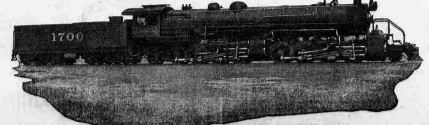
Courtesy Baldwin Locomotive Works, Philadelphia. MALLET TYPE, MODERN LOCOMOTIVE; WEIGHT NEARLY 350 TONS.
