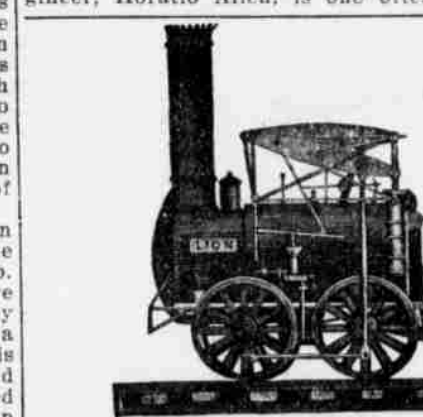
THE STOURBRIDGE LION. First Locomotive to Turn a Wheel in America—Event Occurred at Honesdale, August 8, 1829—Weight, Seven Tons.
