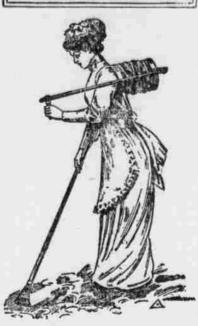
In the hand operated vacuum cleaner herewith illustrated, which has been recently placed on the market, a bellows, strapped to the back and around the waist, provides the suction, says Popular Mechanics. A lever, worked to and fro by the left hand, operates the bellows, and the right hand directs the suction nozzle. The dust is drawn into the bellows, where it is confined by means of porous felt. The apparatus weighs only five and a half pounds
