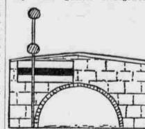
though not the exact proportions is shown in the accompanying drawing On another bridge (six miles away) was mounted a small telescope for sighting. This was placed at exactly the same height as the stripe. Half way between the two was a pole on which were two red disks. four feet apart. The uppermost was adjusted at the same height above the water as the telescope and black stripe. Viewed through the telescope the disks appeared as they do in the drawing.
